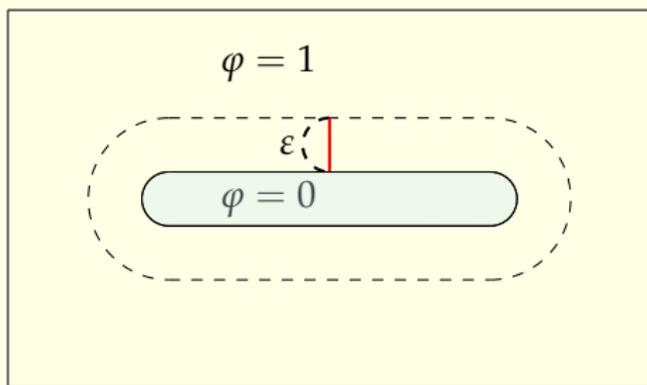
**Figure:** Fracture representation using the phase field  $\varphi$ . The inner blue region indicates the crack with  $\varphi = 0$  and the red region indicates the unbroken zone where  $\varphi = 1$ . We have a diffusive zone in between (green region).
