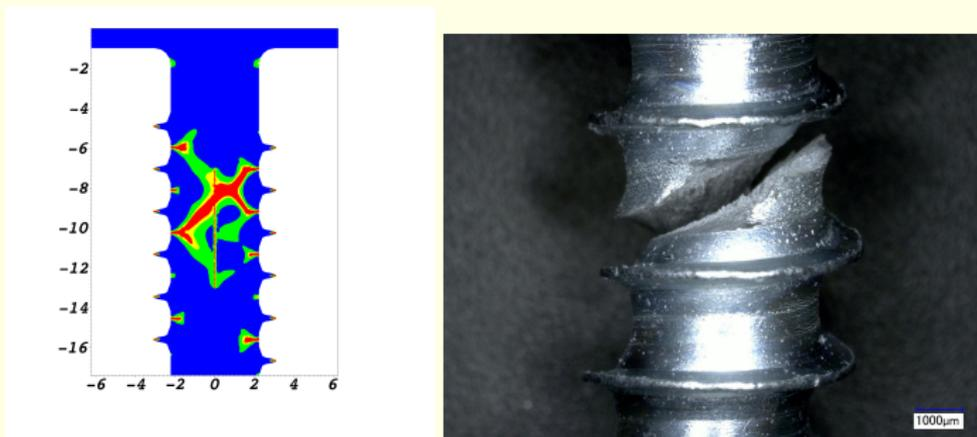
**Figure:** Uniaxial tension and crack nucleation at points with highest stresses. Experimental data from D. Wick (EJOT, Germany).
