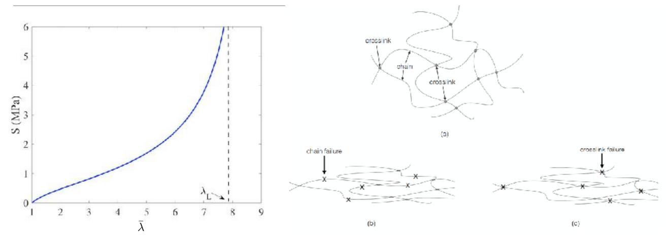
The classical inverse Langevin-type free energy function based on a change in entropy, has a
